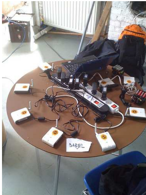
Photo above : Flashed BABEL nodes for mesh networking tests before deployments
